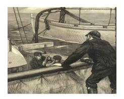
You know the way you measured the water temperature was to simply drop a water bag attached at the end of the rope, drop it to the sea and fill the water bag with sea water.
